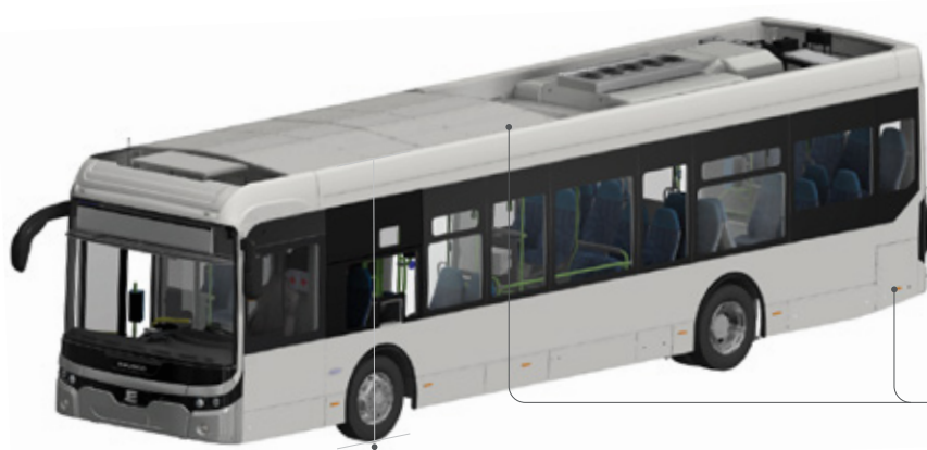
BATTERY PLACEMENT ROOF AND BACK
