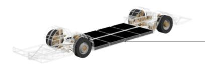
**FULLY FLAT FLOOR**BATTERIES INCORPORATED
